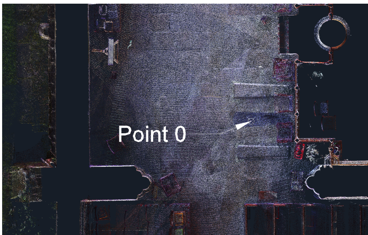
Figure 16. Reference point on the central slab grave cover in the transept, serving as the datum (level 0) for height measurement in this analysis.
