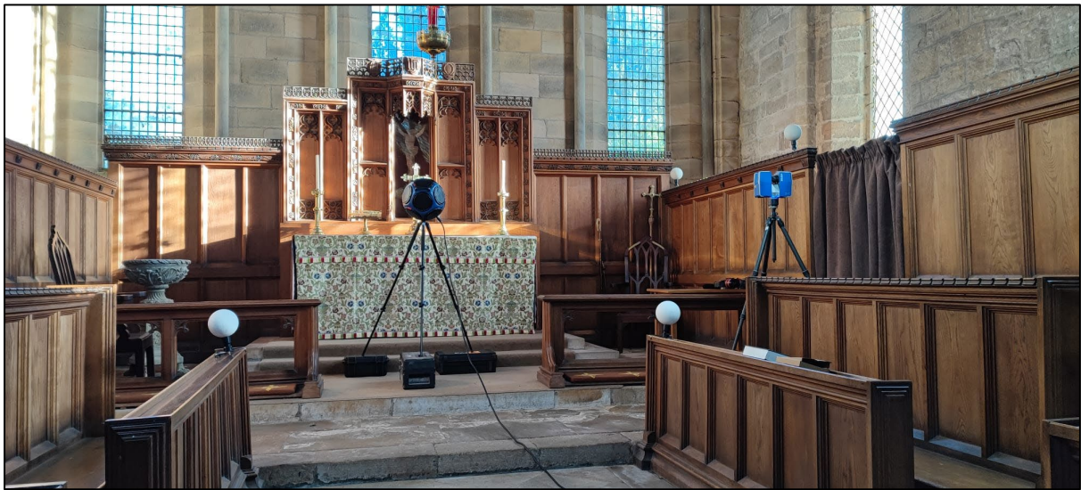
Figure 2. Acoustic test setup and FARO Focus3D X 330 laser scanner. Blanchland, 14 January 2023.
